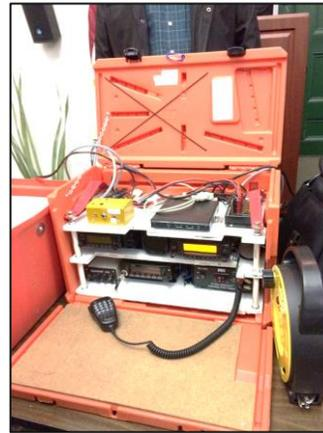
I had previously built an all-thread go box but how nice to meet Norm for his ideas! He used all-thread with small pvc pipe holding each shelf up. There's also a cloth red strap so he can lift the shelf system out of the box. Noticed he notched the shelves for cords? Small details are priceless if we share them.
